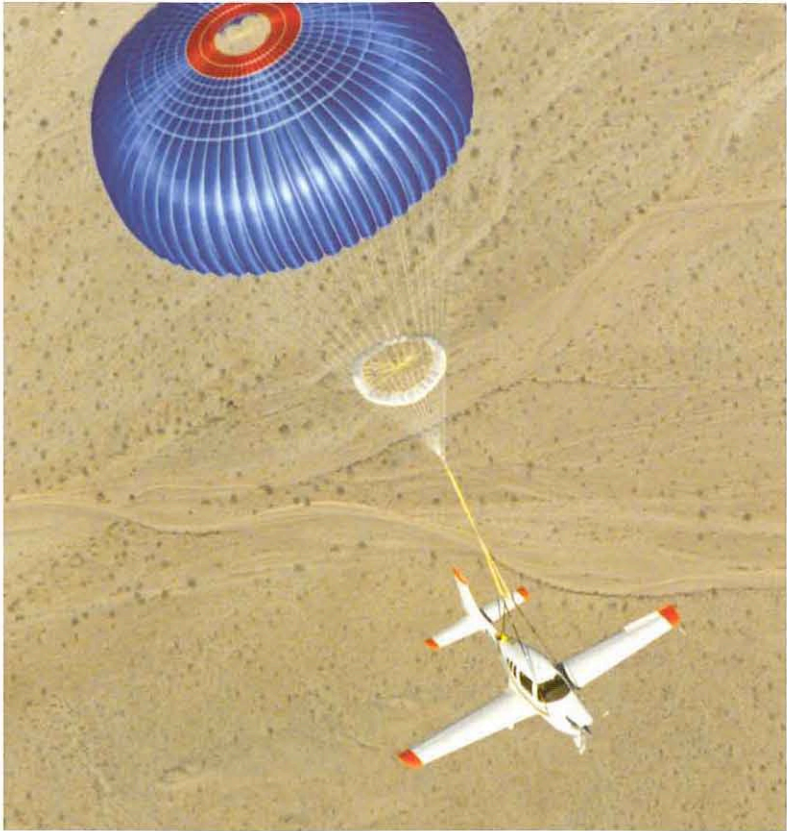
In case of a catastrophic failure, the ballistic recovery system acts as a safety net, enabling the pilot and craft to return safely to earth.
